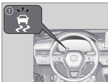
① VSA System Indicator
